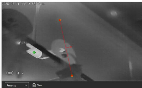
Figure 5-5 Set Single Line Crossing line.
