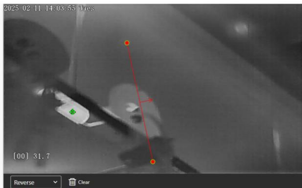
Figure 5-5 Set Single Line Crossing line.
