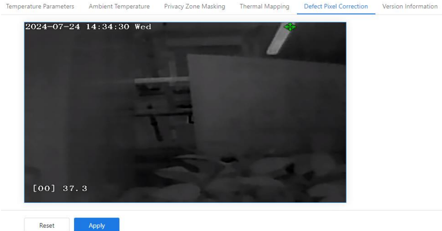
Figure 4-7 Recover Defect Pixel
